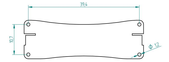
In order to fix the machine, please use properly dowels for the wall where you will place it.
